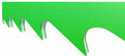
Multiple cutting edges / split chip
